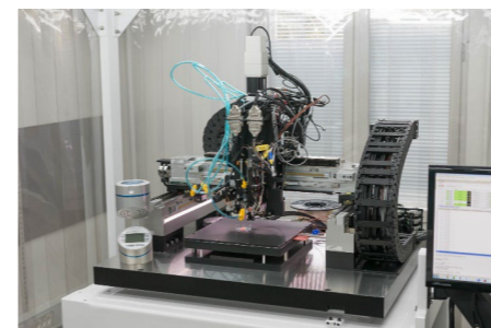
3D polymer printing in clean room
